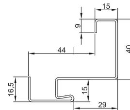
Angle-bar small door frame with a distancing bending on front lapel
