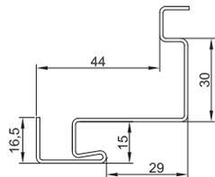
Angle-bar small door frame with separating bending
