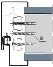
Assembly on plasterboard wall with self-drilling screws [a] (s.c. dry assembly).
