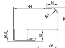
Angle-bar small door frame with a R8 radius on front lapel
