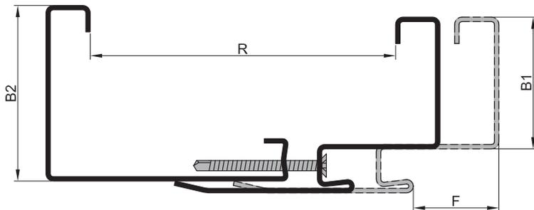
Adjustment of the door frame range up to 25 mm
