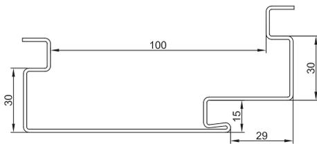
Angle-bar door frame with separating bending
