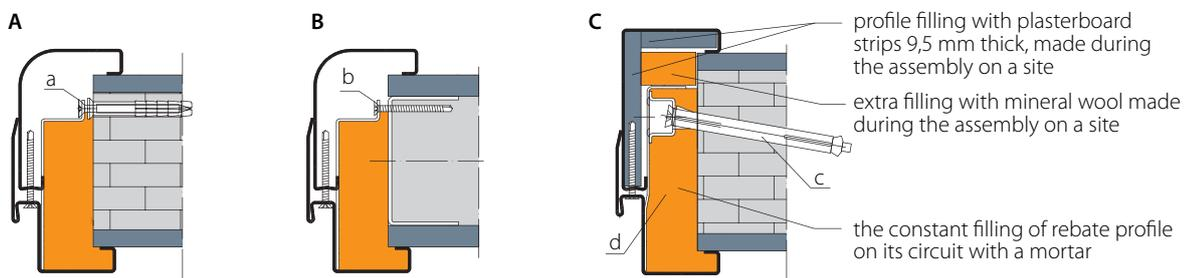
a) assembly on masonry wall with expansion bolts [a] and mounting foam
