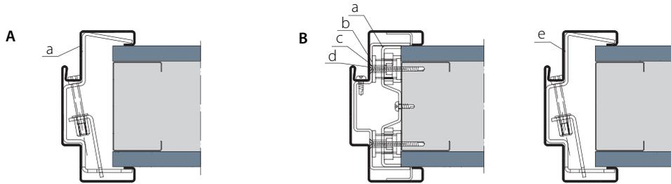
A. Method of anchoring to light door leaves
