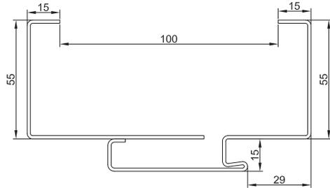
Adjustable PS door frame with sharp edges
